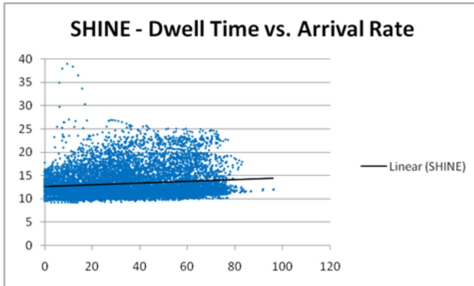
**Figure 35. Correlation of Arrival Rate to SHINE Dwell Time (minutes and flights per hour)**
