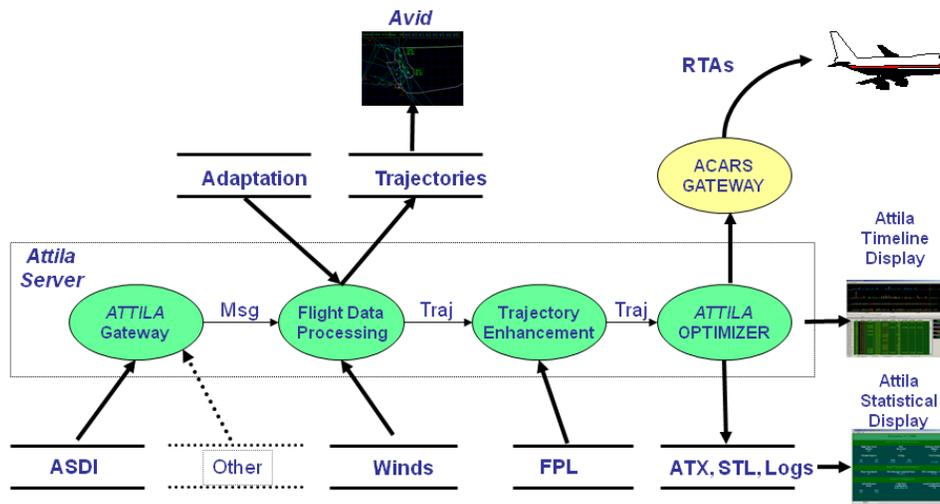
**Figure 3. AAMS Test System Context**
